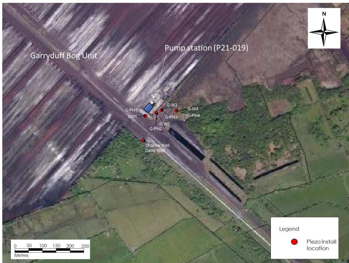
Figure E: Garryduff - piezometer install location map
